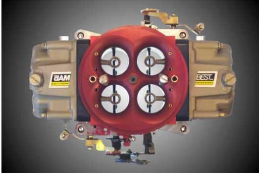
circuits means simple and inexpensive adjustment. At 10" of water it flows 650 CFM; at 20", 933 CFM. Venturi diameter is 1.395". It's recommended for engines of 500 to 750 HP.
