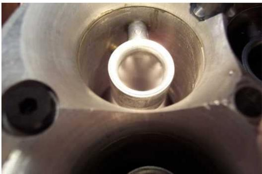
The patent pending design has improved booster signal by 50%, reducing manifold wetting by surrounding the fuel being distributed by the booster with a layer of air to keep fuel off of the walls.
