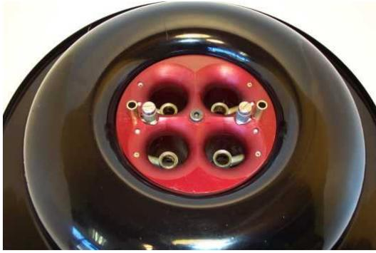
With a 50% increase in booster signal and *dAM's* patented Emulsification System, there is about 50 times the emulsion in previously modified carbs: the droplets are 50 times smaller and there are 50 times more of them.
