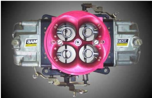
Every effort to improve performance and simplify carb design was made. The carb's billet design allows for custom sizes and lighter weight. This carb flows 1100 CFM at 20" of water. Venturi diameter is 1.585". It's recommended for engines of 700 to 850 HP.
