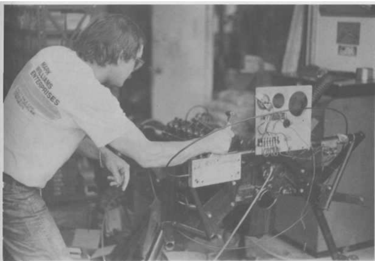
Although it may not look like much, John Satterfield's cylinder head dyno has taken valvetrain science a giant step into the future. By being able to observe the valvetrain in operation, Satterfield (left) can detect any irregularities and then tighten up the weak link.
