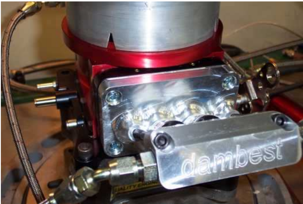
View from end: fuel rail
