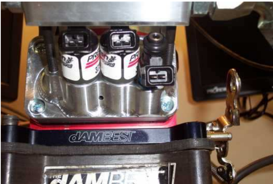
View from below: electronic jets (minus the spacer on the right one)
