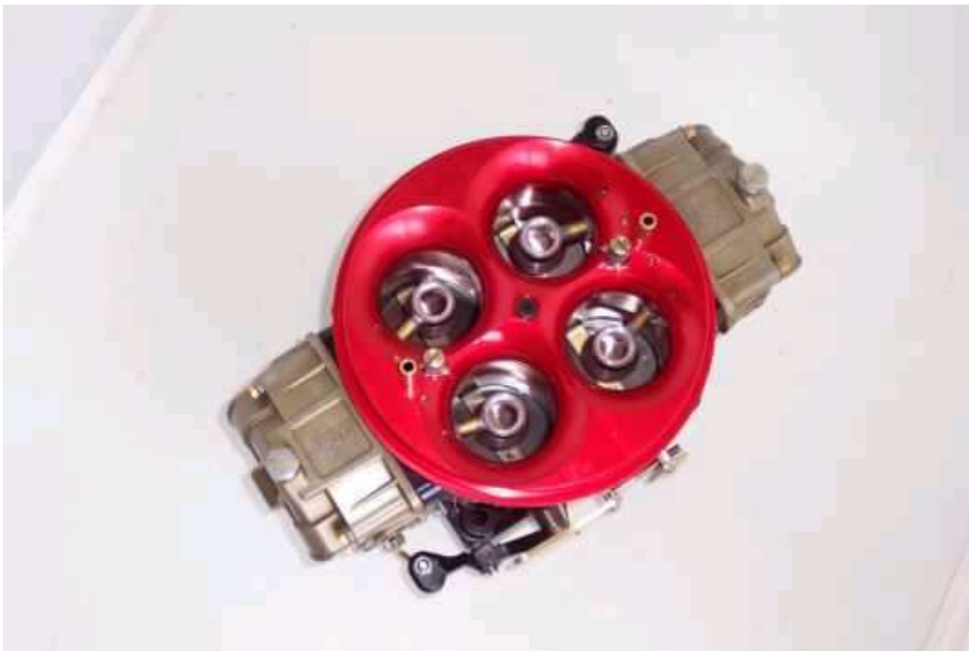
Top View, showing latest booster assemblies. 34" of booster signal at 10" draw on carb, Wow!!!!!!!!!!!!!! Wet flow pictures to follow.
