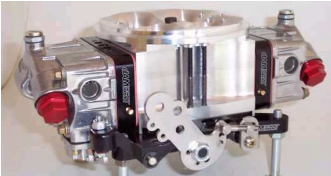
A look at the new linkage for the 4150 style carbs.
