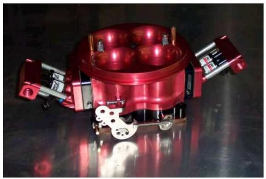
This is a current picture of our 4500-3 with E-Jets installed. Incorporating current patents, along with two more in pending.
