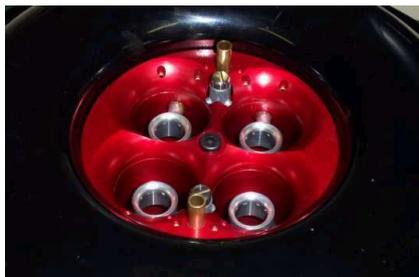
The *dAMBEST* billet carbs are the most powerful and responsive carbs of their size. Every angle of throttle position is adjustable, and adjustable linkage allows control of the rate at which the secondary is applied.
